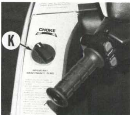
Fig. JS1-7—On JS300SX models, choke knob (K) is located on left side of riding platform and is rotated to control choke plate position.
