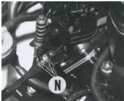
Fig. JS1-13—Rotate locknuts (N) up or down cable housing end as needed to adjust throttle lever free play.
