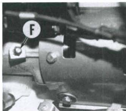
Fig. JS1-1—Intermediate housing is greased through grease fitting (F).
