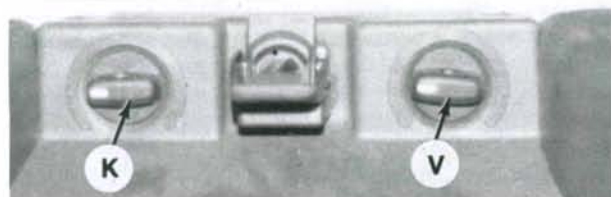
Fig. JS3-2—View identifies location of choke knob (K) and fuel selector valve (V) on JS650SX models.
