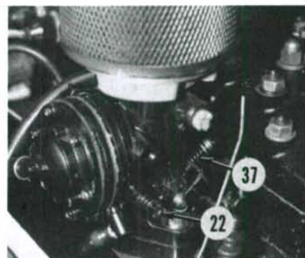
Fig. JS2-6—View identifies location of low speed mixture needle (22) and idle speed screw (37) on JS440 models and JS550 models prior to 1986.
