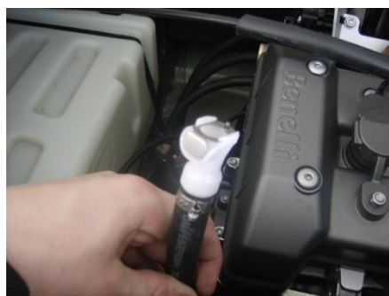
Flushing system fitting
